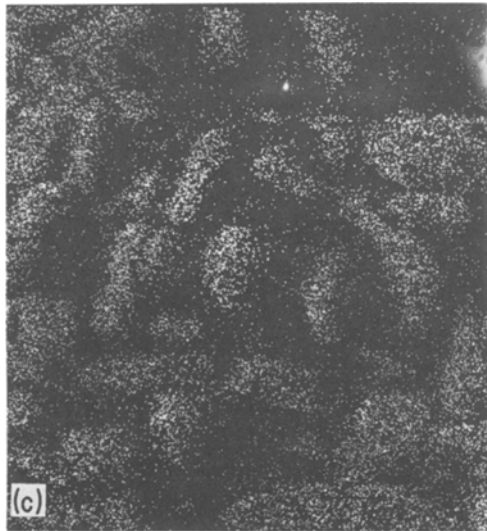
Figure 13 SEMs and WDS map showing concentration of Mg on surface of hot-pressed \text{Si}_3\text{N}_4 specimen doped with 8 wt% \text{Y}_2\text{O}_3 + 1 wt% MgO and oxidized at 1593 K for 30 h. (a) morphology (b) back-scattered electron image, (c) Mg map.
